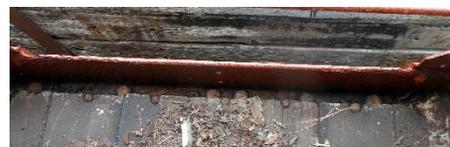
The above 2 photos show the most obvious moisture trap on the brake. There are drainage holes but since 1942 they have slowly filled until they blocked and water rotted away the timber base plates. The timber is on order and Mike will make new ones for fitting soon.
